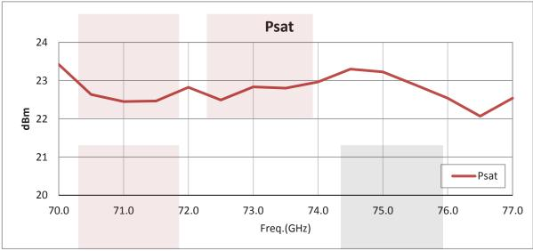
WR-12 Waveguide Power Amplifier 70.5 GHz to 76.5 GHz Frequency Range E Band With 25 dB Gain And 22 dBm Psat Using UG-387/U Flange from Fairview Microwave is in-stock and available to ship same-day. All of our RF/microwave products are available off-the-shelf from our ISO 9001:2008 certified facilities in Allen, Texas. Fairview Microwave is RF on-demand.
