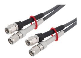
Fairview Microwave's skew matched cables consist of seven models that are extremely flexible and have delay match as low as 1 ps. These cables deliver excellent VSWR of 1.4:1 and are 100% tested for skew match. They also include polarity indicators and restraint bands to keep them paired up.
