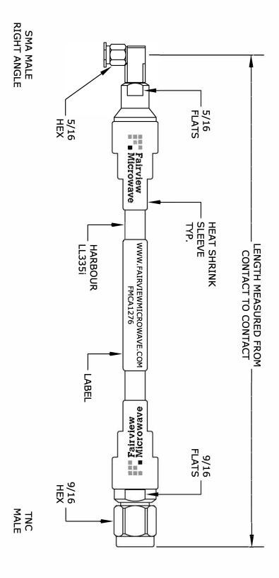
$\overline{\text{NOTE}}$ : LABEL FOR CABLE LENGTHS 48" OR SHORTER TO BE CENTERED . LONGER THAN 48" WILL BE 6" AWAY FROM CONNECTOR .
