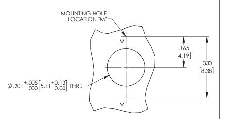
MOUNTING HOLE DETAIL (MOUNTING HARDWARE TO BE DETERMINED BY USER)
