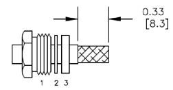
2. FORM BRAID OVER CLAMP NUT (4). TRIM BRAID BACK TO SHOULDER. CUT DIELECTRIC & CENTER CONDUCTOR TO DIMENSION SHOWN. DO NOT NICK CENTER CONDUCTOR. SOLDER CONTACT TO CENTER CONDUCTOR. REMOVE EXCESS SOLDER. DO NOT OVER HEAT DIELECTRIC. INSERT CABLE ASSEMBLY INTO BODY & TIGHTEN.
