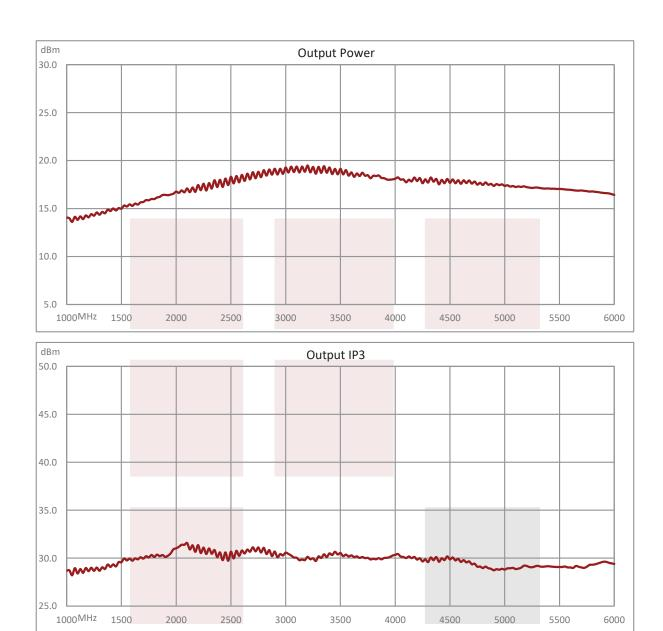
1.0 dB NF Low Noise Amplifier, Operating from 1 GHz to 6 GHz with 18 dB Gain, 18.5 dBm P1dB and SMA from Fairview Microwave is in-stock and available to ship same-day. All of our RF/microwave products are available off-the-shelf from our ISO 9001:2008 certified facilities in Lewisville, Texas. Fairview Microwave is RF on-demand.
