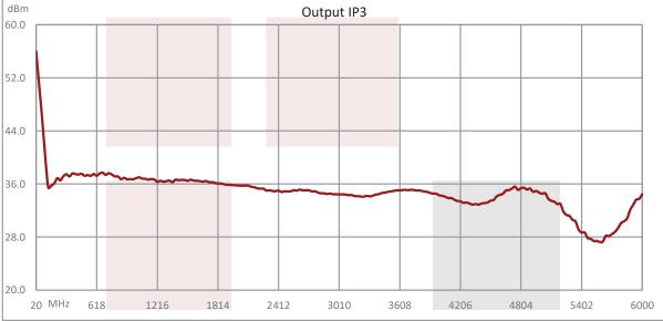
2.0 dB NF Low Noise Amplifier, Operating from 20 MHz to 6 GHz with 59 dB Gain, 18 dBm P1dB and SMA from Fairview Microwave is in-stock and available to ship same-day. All of our RF/microwave products are available off-the-shelf from our ISO 9001:2008 certified facilities in Lewisville, Texas. Fairview Microwave is RF on-demand.
