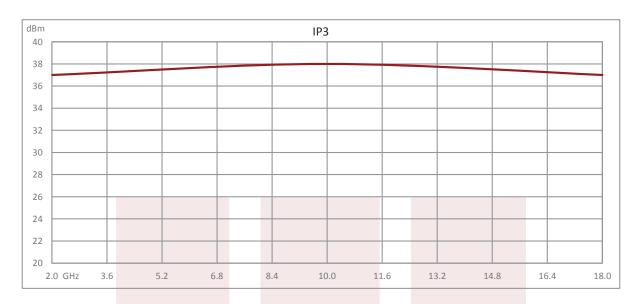
Medium Power Amplifier at 1 Watt P1dB Operating from 2 GHz to 18 GHz with 37 dBm IP3, SMA from Fairview Microwave is in-stock and available to ship same-day. All of our RF/microwave products are available off-the-shelf from our ISO 9001:2008 certified facilities in Allen, Texas. Fairview Microwave is RF on-demand.
