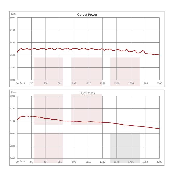
1 Watt P1dB, 30 MHz to 2200 MHz, Medium Power GaAs Amplifier with Heatsink, 31 dB Gain, 43 dBm IP3 and SMA from Fairview Microwave is in-stock and available to ship same-day. All of our RF/microwave products are available off-the-shelf from our ISO 9001:2008 certified facilities in Lewisville, Texas. Fairview Microwave is RF on-demand.
