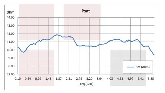
60 dB Gain High Power High Gain Amplifier at 10 Watt Psat Operating from 100 MHz to 6 GHz with SMA from Fairview Microwave is in-stock and available to ship same-day. All of our RF/microwave products are available off-the-shelf from our ISO 9001:2008 certified facilities in Lewisville, Texas. Fairview Microwave is RF on-demand.
