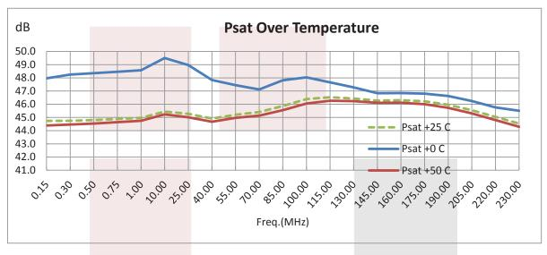
43 dB Gain High Power High Gain Amplifier at 25 Watt Psat Operating From 0.15 MHz to 230 MHz with 48 dBm IP3 and SMA from Fairview Microwave is in-stock and available to ship same-day. All of our RF/microwave products are available off-the-shelf from our ISO 9001:2008 certified facilities in Allen, Texas. Fairview Microwave is RF on-demand.
