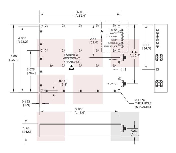
NOTE: HEAT SINK REQUIRED FOR PROPER OPERATION, UNIT IS COOLED BY CONDUCTING TO HEAT SINK.
