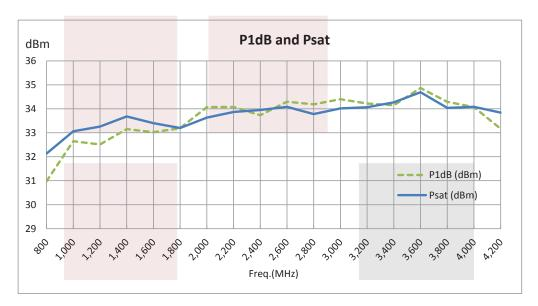
Medium Power GaAs Amplifier at 1.5 Watt Psat Operating from 800 MHz to 4.2 GHz with 41 dBm IP3, SMA from Fairview Microwave is in-stock and available to ship same-day. All of our RF/microwave products are available off-the-shelf from our ISO 9001:2008 certified facilities in Lewisville, Texas. Fairview Microwave is RF on-demand.
