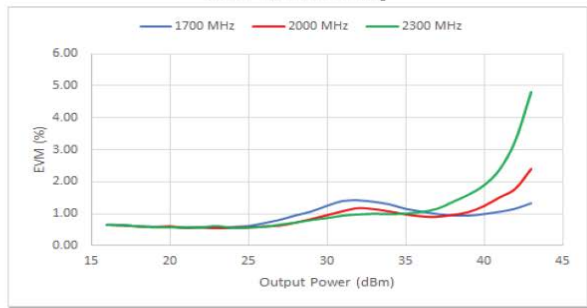
Error Vector Magnitude vs. Output Power [64QAM, 5Msps, 10% Roll Off Rate]
