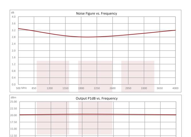
35 dB min Gain, Temperature Compensated Low Noise Amplifier, 21 dBm P1dB Operating from 0.5 GHz to 4 GHz with SMA and Heatsink from Fairview Microwave is in-stock and available to ship same-day. All of our RF/microwave products are available off-the-shelf from our ISO 9001:2008 certified facilities in Lewisville, Texas. Fairview Microwave is RF on-demand.
