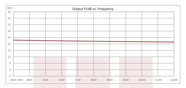
35 dB min Gain, Temperature Compensated Low Noise Amplifier, 22 dBm P1dB Operating from 4 GHz to 12 GHz with SMA and Heatsink from Fairview Microwave is in-stock and available to ship same-day. All of our RF/microwave products are available off-the-shelf from our ISO 9001:2008 certified facilities in Lewisville, Texas. Fairview Microwave is RF on-demand.
