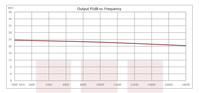
35 dB min Gain, Temperature Compensated Low Noise Amplifier, 20 dBm P1dB Operating from 2 GHz to 18 GHz with SMA and Heatsink from Fairview Microwave is in-stock and available to ship same-day. All of our RF/microwave products are available off-the-shelf from our ISO 9001:2008 certified facilities in Lewisville, Texas. Fairview Microwave is RF on-demand.
