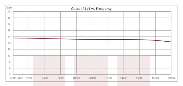
35 dB min Gain, Temperature Compensated Low Noise Amplifier, 20 dBm P1dB Operating from 6 GHz to 18 GHz with SMA from Fairview Microwave is in-stock and available to ship same-day. All of our RF/microwave products are available off-the-shelf from our ISO 9001:2008 certified facilities in Lewisville, Texas. Fairview Microwave is RF on-demand.
