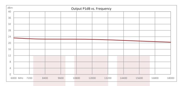
35 dB min Gain, Temperature Compensated Low Noise Amplifier, 20 dBm P1dB Operating from 6 GHz to 18 GHz with SMA and Heatsink from Fairview Microwave is in-stock and available to ship same-day. All of our RF/microwave products are available off-the-shelf from our ISO 9001:2008 certified facilities in Lewisville, Texas. Fairview Microwave is RF on-demand.
