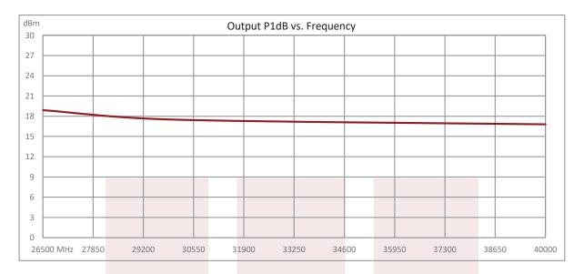
35 dB min Gain, Temperature Compensated Low Noise Amplifier, 18 dBm P1dB Operating from 26.5 GHz to 40 GHz with 2.92mm from Fairview Microwave is in-stock and available to ship same-day. All of our RF/microwave products are available off-the-shelf from our ISO 9001:2008 certified facilities in Lewisville, Texas. Fairview Microwave is RF on-demand.
