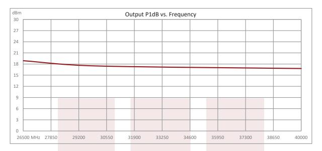
35 dB min Gain, Temperature Compensated Low Noise Amplifier, 18 dBm P1dB Operating from 26.5 GHz to 40 GHz with 2.92mm and Heatsink from Fairview Microwave is in-stock and available to ship same-day. All of our RF/microwave products are available off-the-shelf from our ISO 9001:2008 certified facilities in Lewisville, Texas. Fairview Microwave is RF ondemand.
