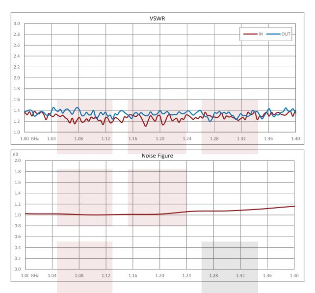
1.2 dB NF Input Protected Low Noise Amplifier, Operating from 1 GHz to 1.4 GHz with 30 dB Gain, 10 dBm P1dB and SMA from Fairview Microwave is in-stock and available to ship same-day. All of our RF/microwave products are available off-the-shelf from our ISO 9001:2008 certified facilities in Allen, Texas. Fairview Microwave is RF on-demand.
