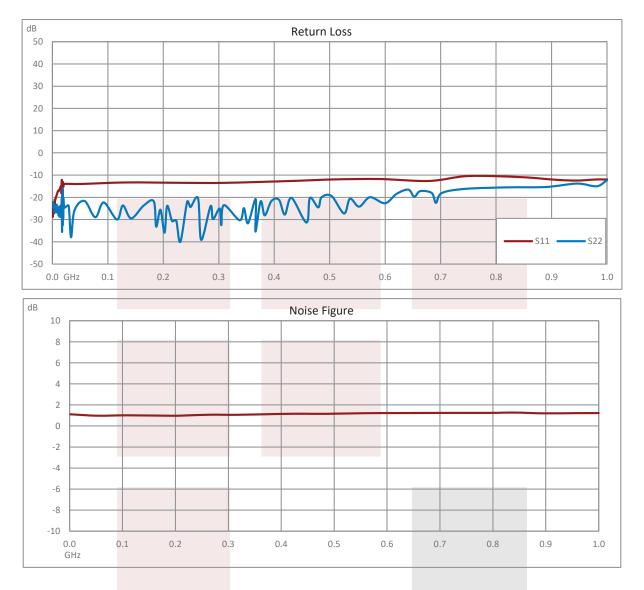
1 dB NF Input Protected Low Noise Amplifier, Operating from 0.001 MHz to 1 GHz with 50 dB Gain, 15 dBm P1dB and SMA from Fairview Microwave is in-stock and available to ship same-day. All of our RF/microwave products are available off-the-shelf from our ISO 9001:2008 certified facilities in Lewisville, Texas. Fairview Microwave is RF on-demand.
