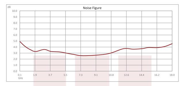
3.5 dB NF Input Protected Low Noise Amplifier, Operating from 100 MHz to 18 GHz with 33 dB Gain, 25 dBm Psat and SMA from Fairview Microwave is in-stock and available to ship same-day. All of our RF/microwave products are available off-the-shelf from our ISO 9001:2008 certified facilities in Lewisville, Texas. Fairview Microwave is RF on-demand.
