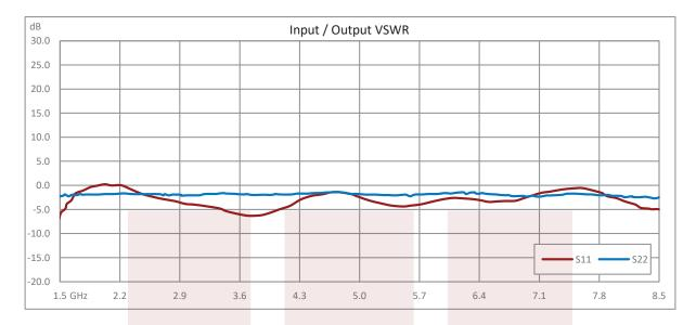
Variable Gain Control Amplifier, 2 GHz to 8 GHz, GaAs FET, 40 dB Gain, 20 dB Variable Gain, +15 dBm P1dB, SMA from Fairview Microwave is in-stock and available to ship same-day. All of our RF/microwave products are available off-the-shelf from our ISO 9001:2008 certified facilities in Lewisville, Texas. Fairview Microwave is RF on-demand.
