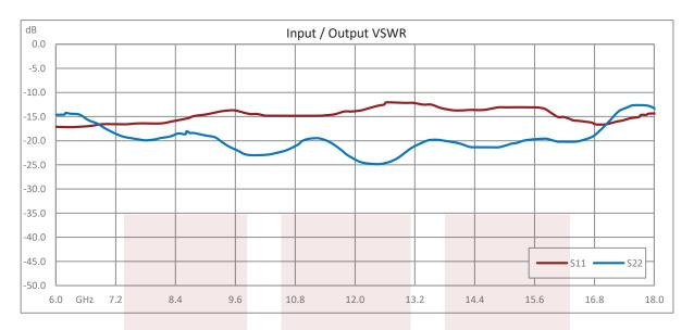
Variable Gain Control Amplifier, 6 GHz to 18 GHz, GaAs FET, 40 dB Gain, 20 dB Variable Gain, +15 dBm P1dB, SMA from Fairview Microwave is in-stock and available to ship same-day. All of our RF/microwave products are available off-the-shelf from our ISO 9001:2008 certified facilities in Lewisville, Texas. Fairview Microwave is RF on-demand.
