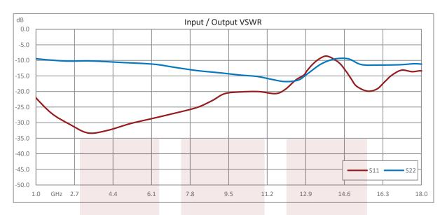
Variable Gain Control Amplifier, 1 GHz to 18 GHz, GaAs FET, 40 dB Gain, 20 dB Variable Gain, +13 dBm P1dB, SMA from Fairview Microwave is in-stock and available to ship same-day. All of our RF/microwave products are available off-the-shelf from our ISO 9001:2008 certified facilities in Lewisville, Texas. Fairview Microwave is RF on-demand.
