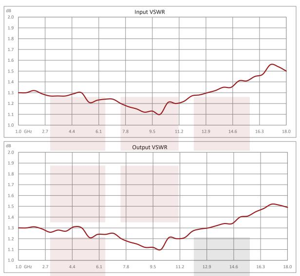
1 GHz to 18 GHz Field Replaceable SMA Positive Slope Equalizer, Max Pin +30, 1.5 dB Loss and 8 Fixed Equalizing Value from Pasternack Enterprises has same day shipment for domestic and International orders Our RF, microwave and millimeter wave products maintain a 99.4% availability and are part of the broadest selection in the industry.
