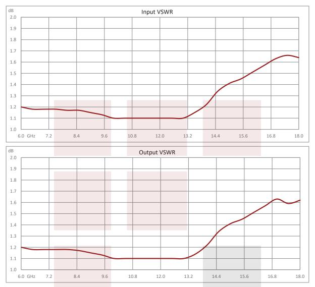
6 GHz to 18 GHz Field Replaceable SMA Positive Slope Equalizer, Max Pin +30, 1.5 dB Loss and 4 Fixed Equalizing Value from Pasternack Enterprises has same day shipment for domestic and International orders Our RF, microwave and millimeter wave products maintain a 99.4% availability and are part of the broadest selection in the industry.
