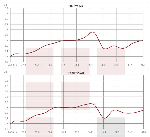
26.5 GHz to 40 GHz Field Replaceable 2.92mm Positive Slope Equalizer, Max Pin +30, 2.5 dB Loss and 5 Fixed Equalizing Value from Pasternack Enterprises has same day shipment for domestic and International orders Our RF, microwave and millimeter wave products maintain a 99.4% availability and are part of the broadest selection in the industry.
