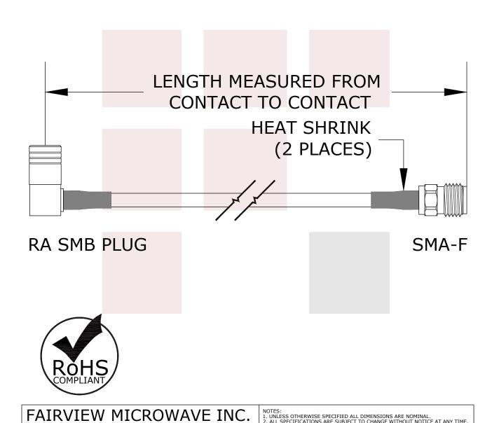
SMA Female to RA SMB Plug Cable RG-316 Coax in 60
