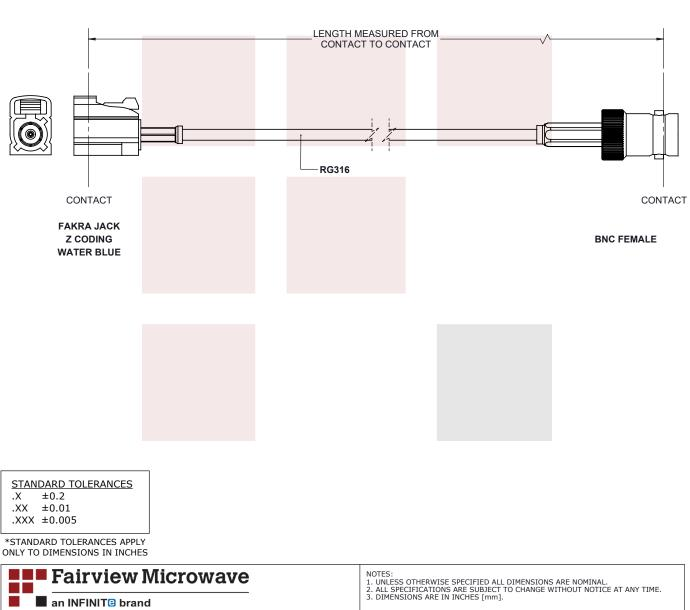
Water Blue FAKRA Jack to BNC Female Cable Using RG316 Coax
