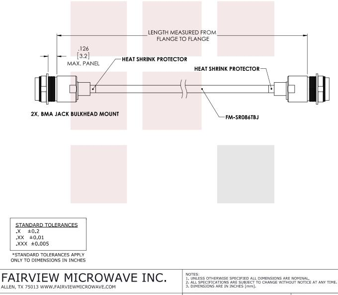
Slide-On BMA Jack Bulkhead to Slide-On BMA Jack Bulkhead Cable FM-SR086TBJ Coax
