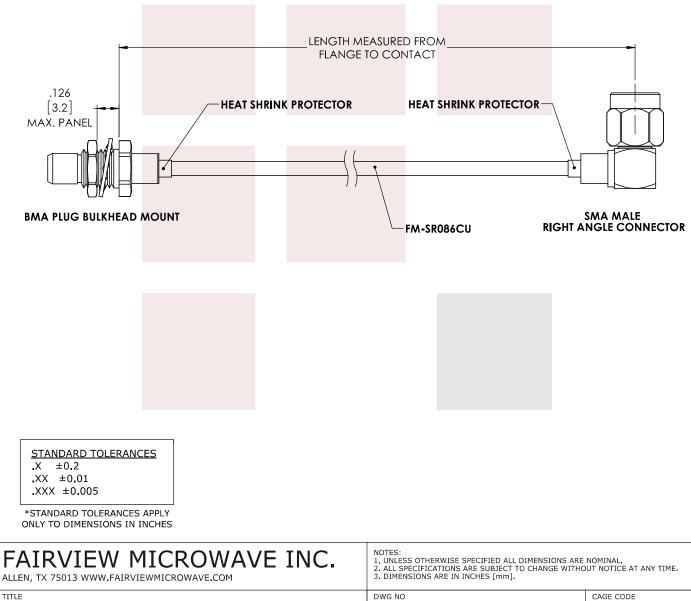
Slide-On BMA Plug Bulkhead to RA SMA Male Cable RG405 Type .086 Coax in 36 Inch
