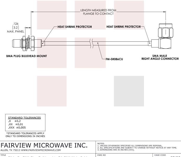
Slide-On BMA Plug Bulkhead to RA SMA Male Cable RG405 Type .086 Coax
