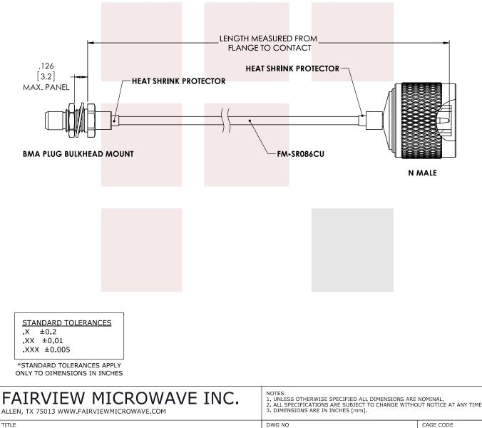
Slide-On BMA Plug Bulkhead to N Male Cable RG405 Type .086 Coax
