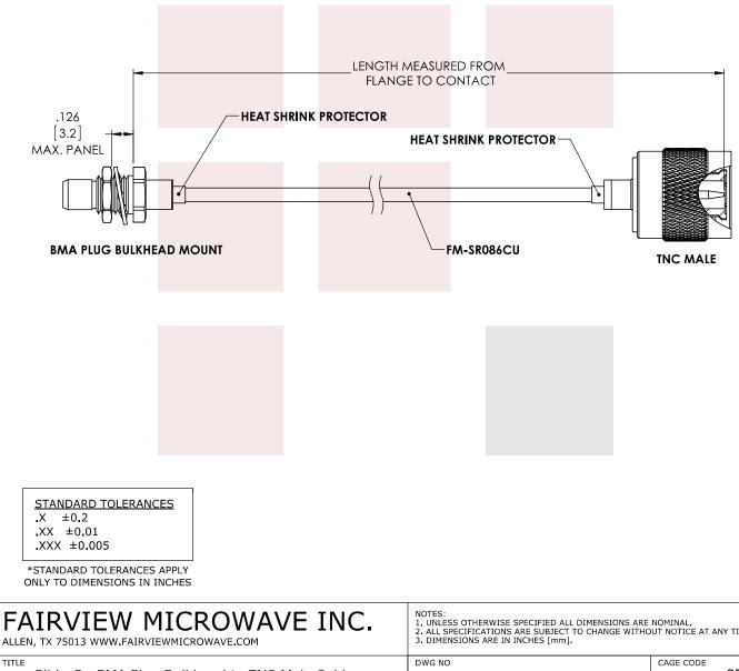
Slide-On BMA Plug Bulkhead to TNC Male Cable RG405 Type .086 Coax
