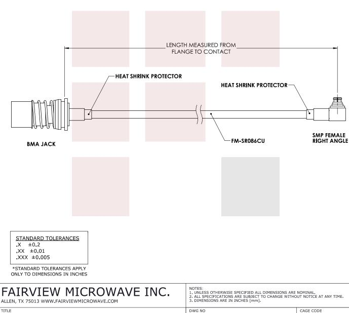
Snap-On BMA Jack to RA SMP Female Cable RG405 Type .086 Coax in 60 Inch
