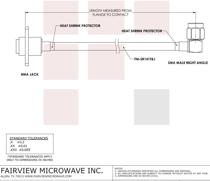
Slide-On BMA Jack 2 Hole Flange to RA SMA Male Cable FM-SR141TBJ Coax in 36 Inch
