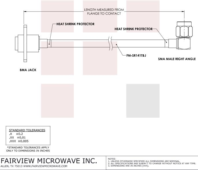
Slide-On BMA Jack 2 Hole Flange to RA SMA Male Cable FM-SR141TBJ Coax in 6 Inch
