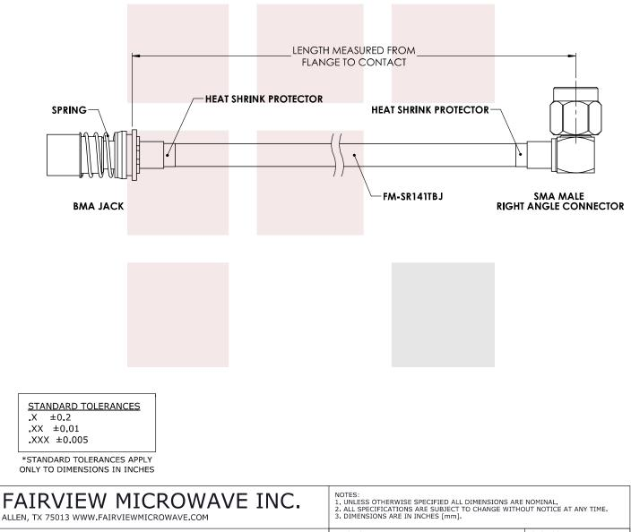
Snap-On BMA Jack to RA SMA Male Cable FM-SR141TBJ Coax in 6 Inch
