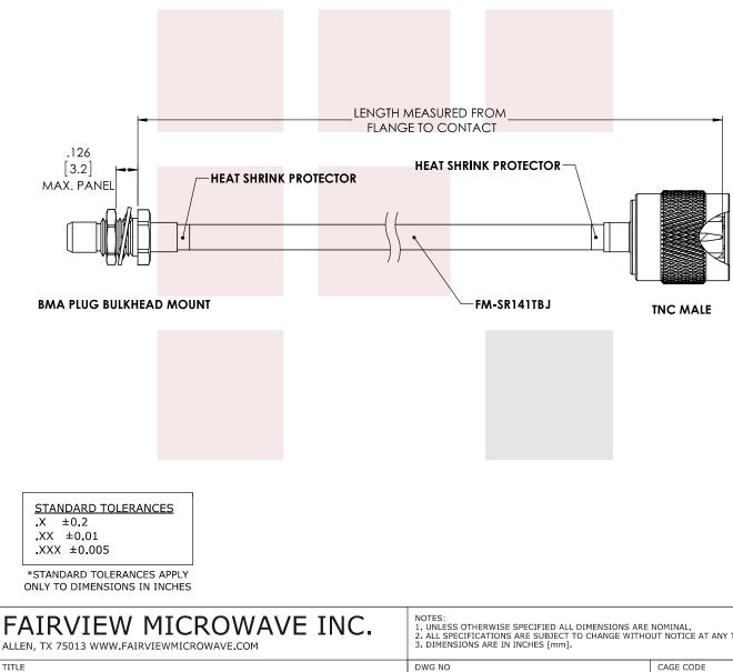
Slide-On BMA Plug Bulkhead to TNC Male Cable FM-SR141TBJ Coax
