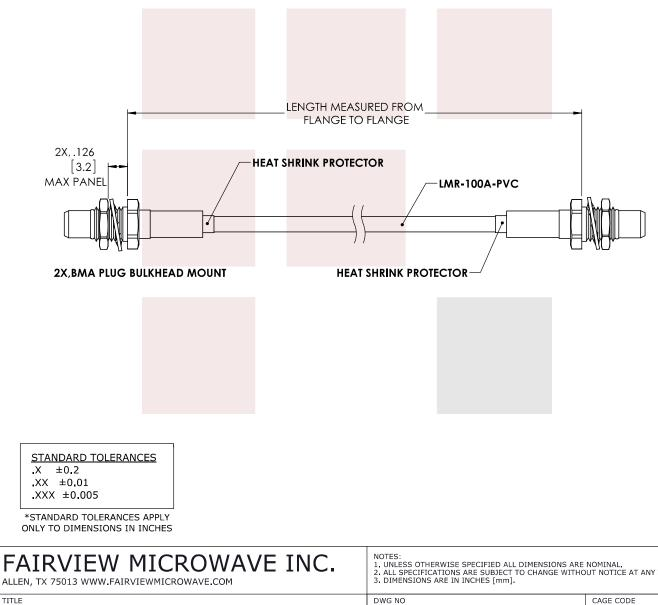
Slide-On BMA Plug Bulkhead to Slide-On BMA Plug Bulkhead Cable LMR-100 Coax in 24 Inch
