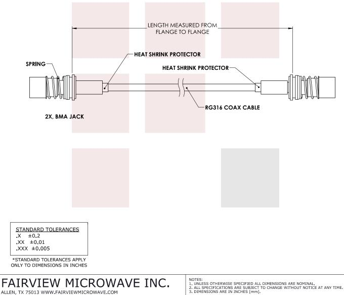
Snap-On BMA Jack to Snap-On BMA Jack Cable RG-316 Coax in 60 Inch
