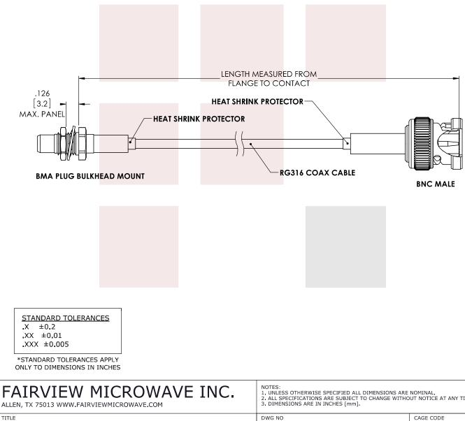
Slide-On BMA Plug Bulkhead to BNC Male Cable RG-316 Coax in 24 Inch
