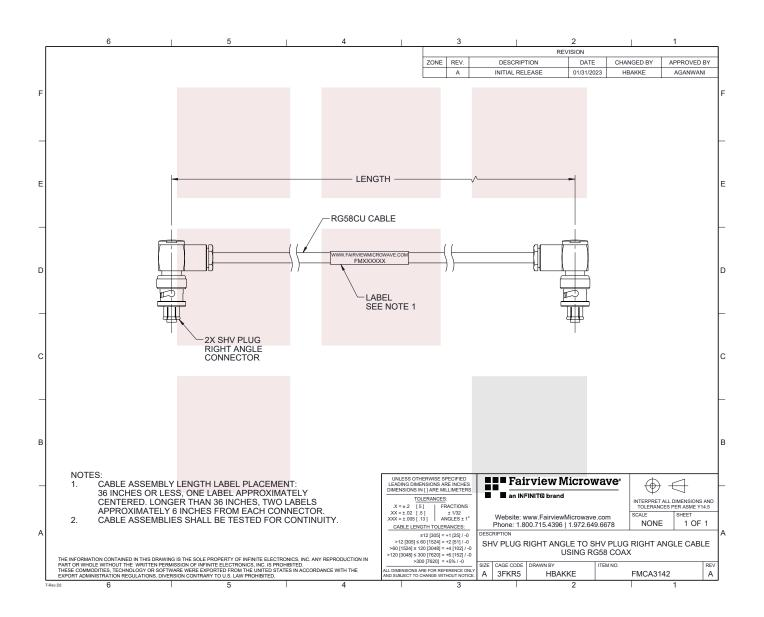
RA SHV Plug to RA SHV Plug Cable RG-58 Coax
