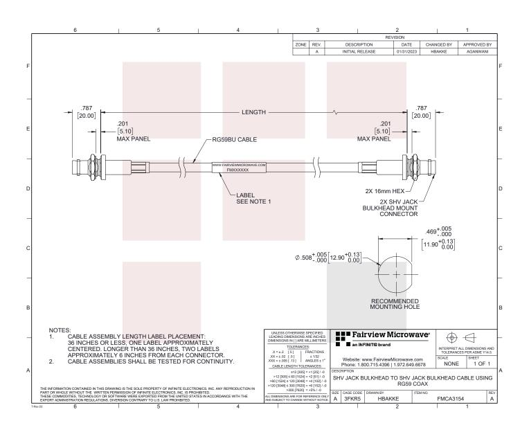
SHV Jack Bulkhead to SHV Jack Bulkhead Cable 75 Ohm RG59 Black Coax
