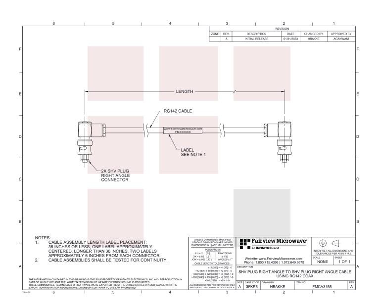
RA SHV Plug to RA SHV Plug Cable RG-142 Coax
