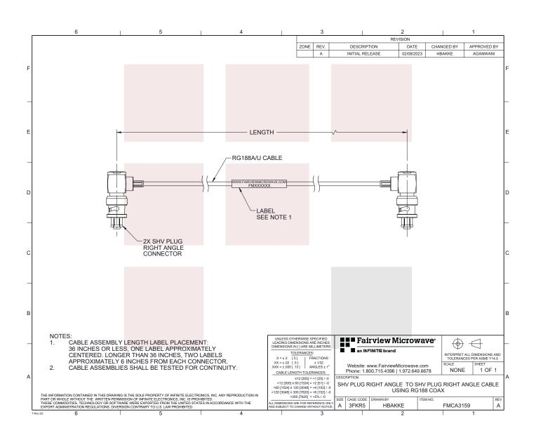
RA SHV Plug to RA SHV Plug Cable RG188 Coax
