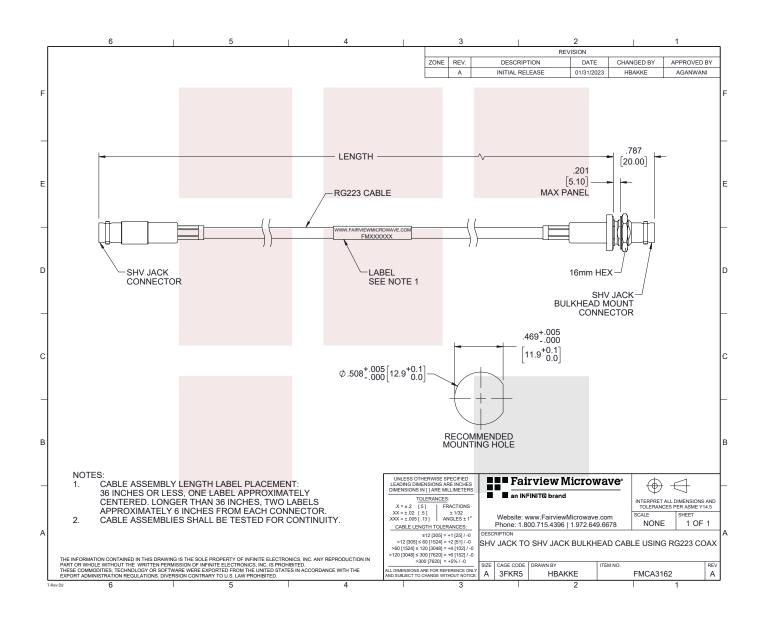
SHV Jack to SHV Jack Bulkhead Cable RG223 Coax in 12 Inch
